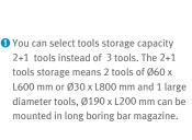
Ø30 x L800 mm sized tool is not Long boring bar but Gun drill. We do not recommend long boring bar sized Ø30 x L800 mm.
